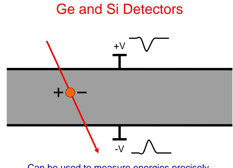
Can be used to measure energies precisely, or positions precisely, or both.
