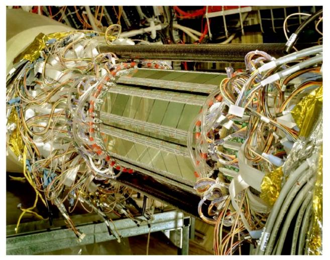
Used to measure charged-particle positions to a few thousandths of an inch.
