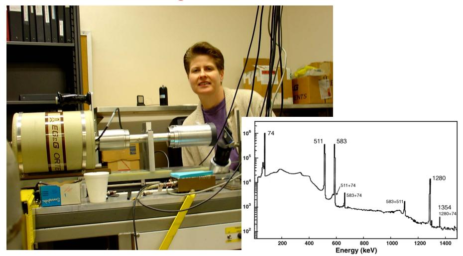
The most precisely calibrated Ge detector in the world is at Texas A&M.
