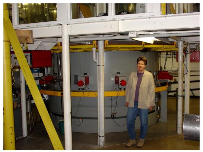
The Texas A&M K500 Superconducting Cyclotron -- can accelerate alpha particles to 280 MeV and uranium over 2000 MeV (40% and 14% of the speed of light, respectively) Sat Morn Physics
