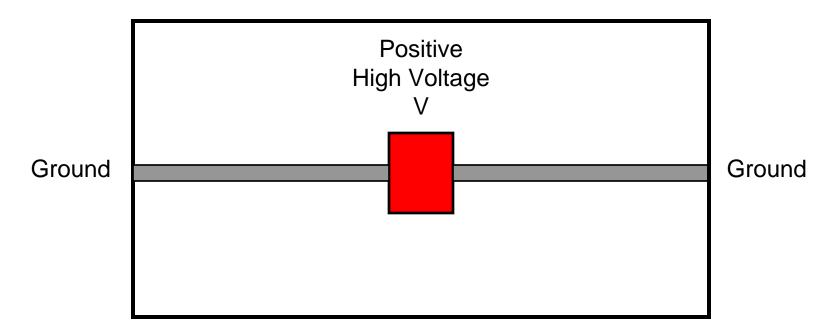
Can achieve energies of 10's of millions of electron volts (MeV), or velocities up to 20% of the speed of light
